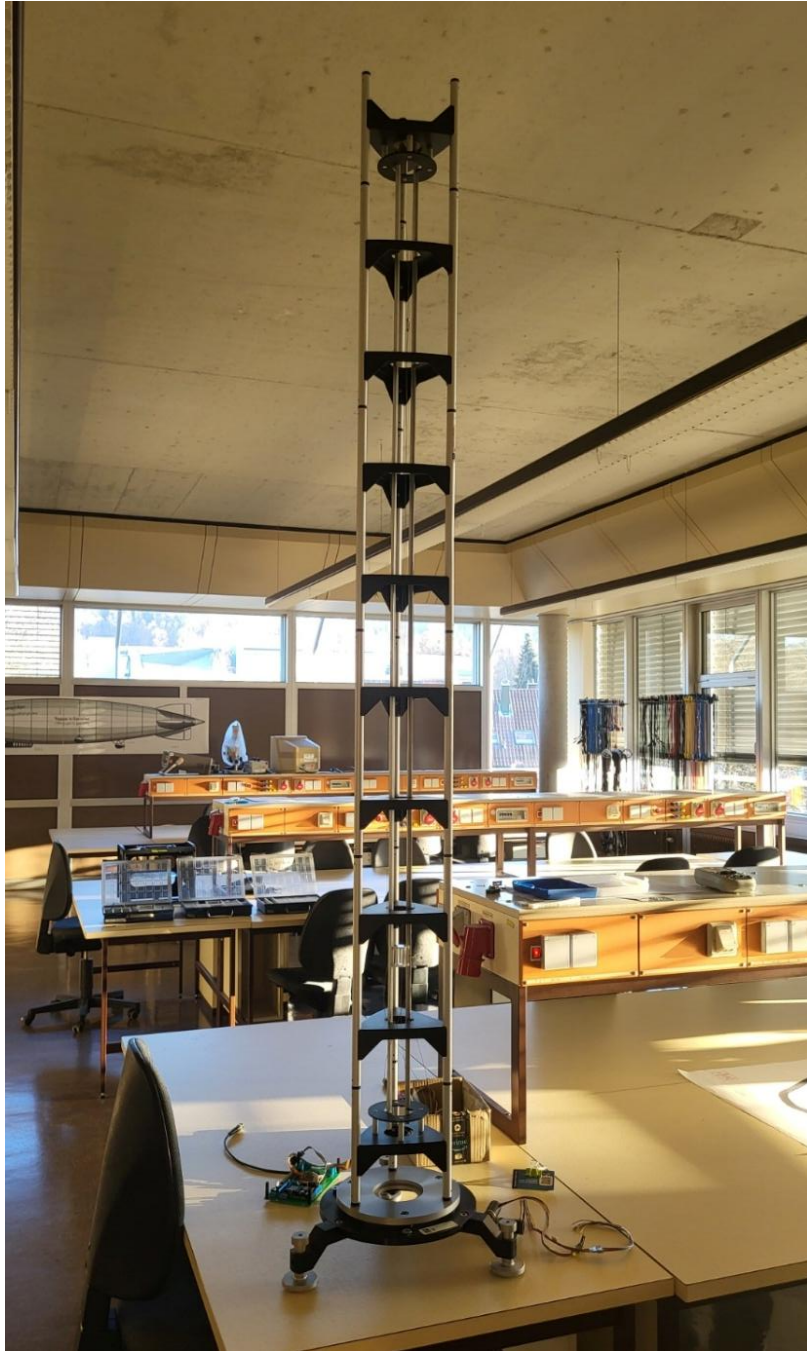
Photo: Mini drop tower in the electronics lab of RWU in Weingarten
